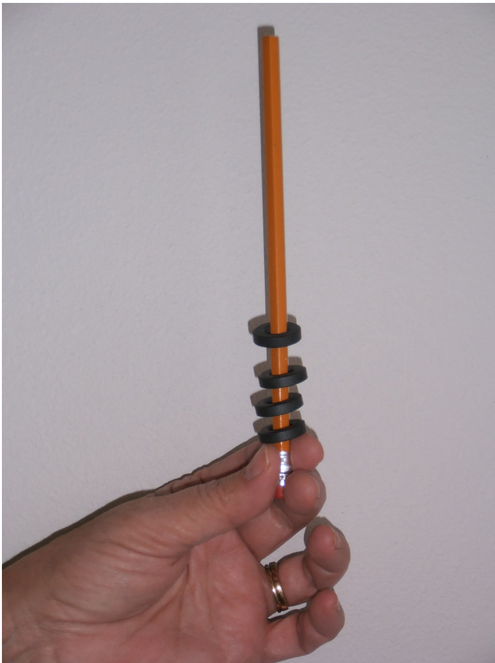
Donut magnets on a post “repelling.”
